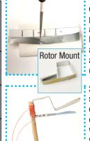
1. Cut a 3½" x ¼" strip of tin, according to the picture. Lay the strip on a folded paper towel. Make two punctures with an awl. Bend the strip as shown in the picture (rotor mount).
